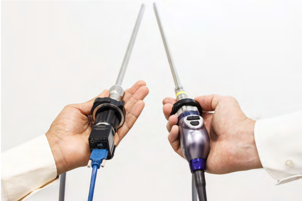
Figure 7.1: The video-rate multispectral laparoscope (left), compared to a standard RGB laparoscope (right).
