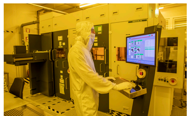
NIL HV equipment in imec's class 1 Fab
